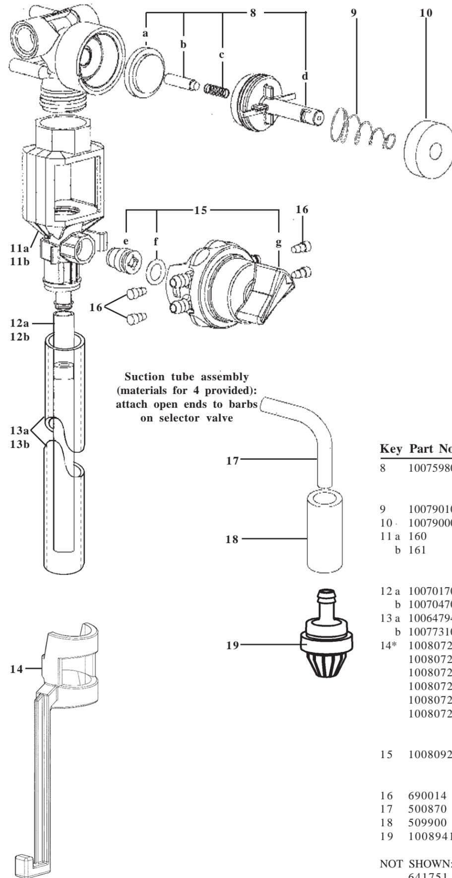
Suction tube assembly (materials for 4 provided): attach open ends to barbs on selector valve
