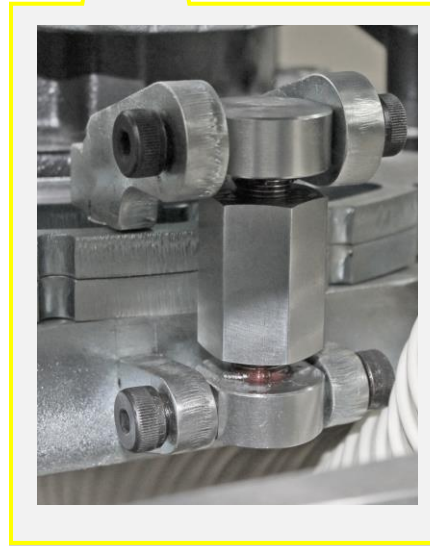
Grinding Head Leveling Adjustment Nut shown adjusted in a AFT position depicted by adjustment nut in a compressed position.
