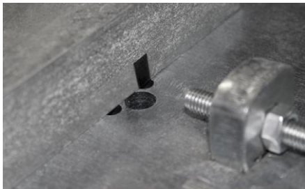
Grinding Head position full RIGHT (black line aligned with right black notch mark)
