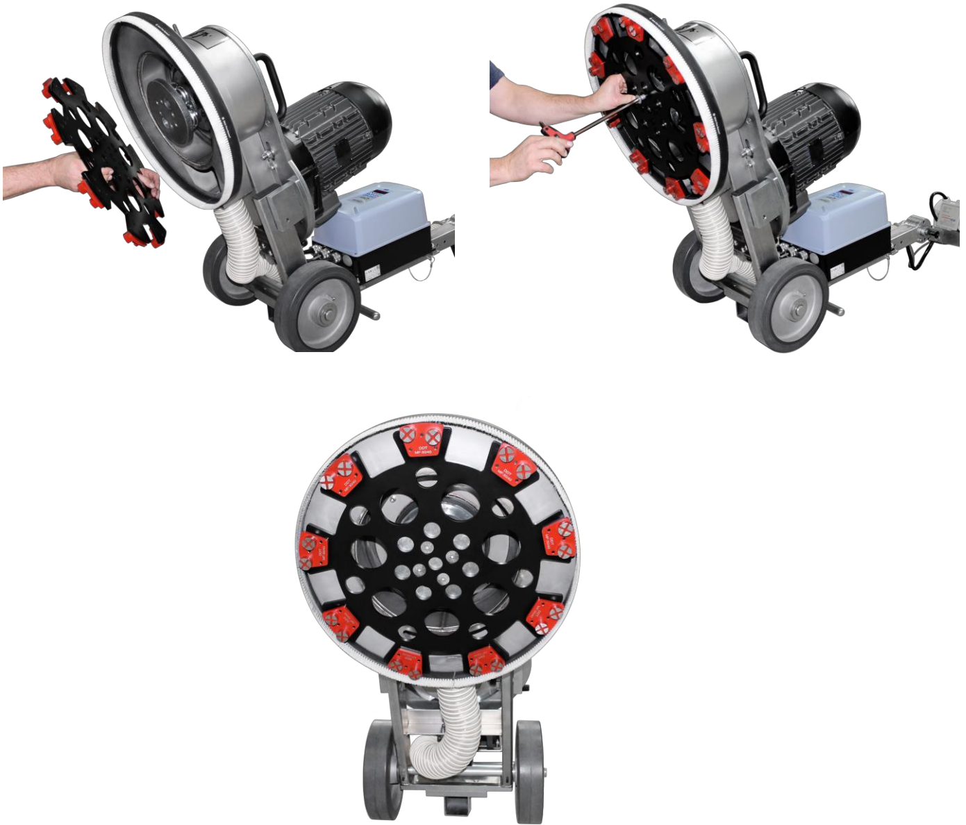
Figure 5-4 How to install a 20" grinding plate to the bottom plate of the machine
