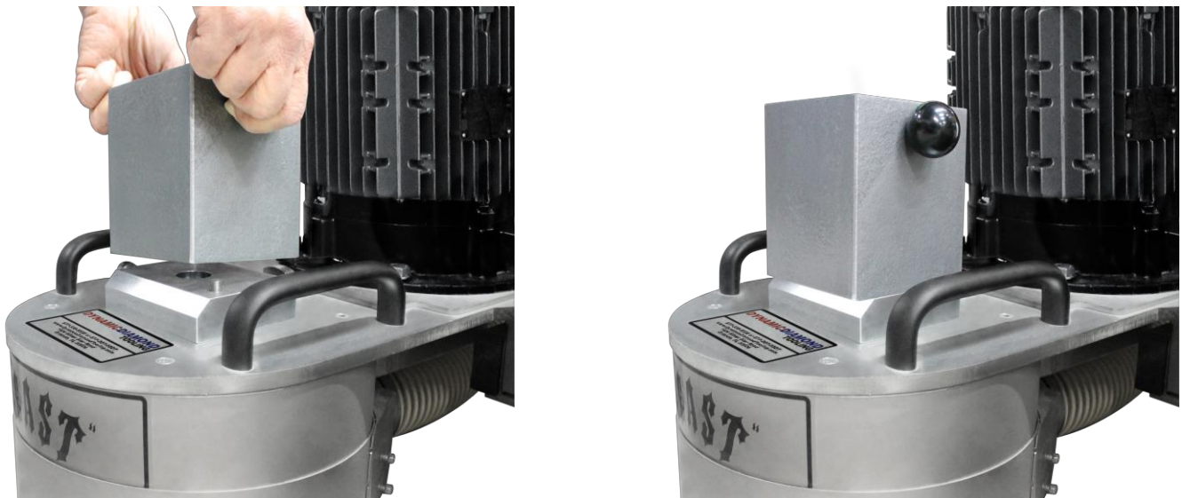
Figure 4-1 How to install additional weight to the head of the machine
