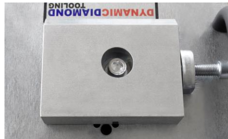
Grinding Head position full RIGHT (black line aligned with right black notch mark)
