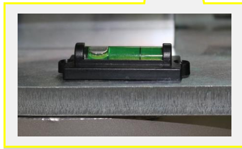
Grinding Head shown in an AFT tilt position depicted by level bubble in FWD position.
