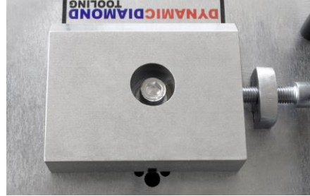
Grinding Head position CENTERED (black line aligned with hole)
