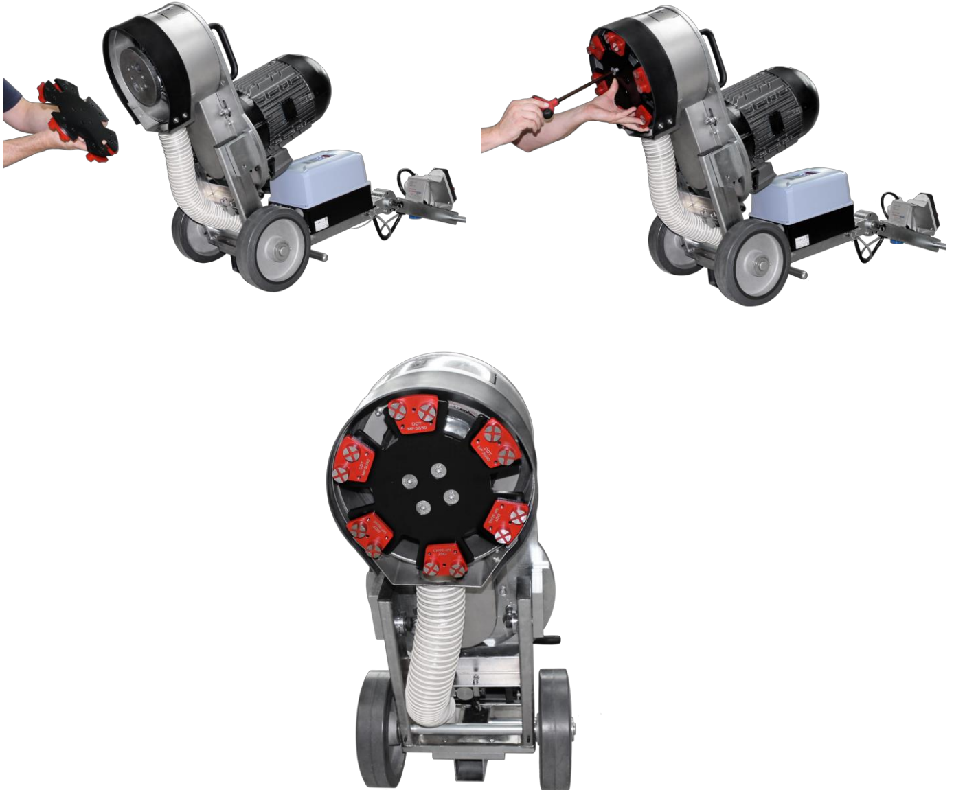
Figure 5-2 How to install a 12” grinding plate to the bottom plate of the machine
