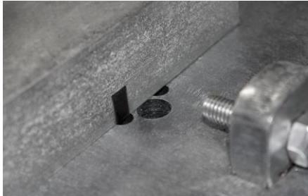
Grinding Head position full LEFT (black line aligned with left black notchmark)
