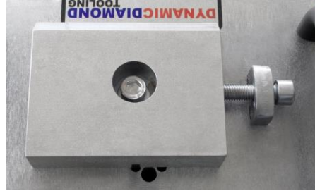
Grinding Head position full LEFT (black line aligned with left black notchmark)
