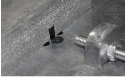
Grinding Head position CENTERED (black line aligned with hole)
