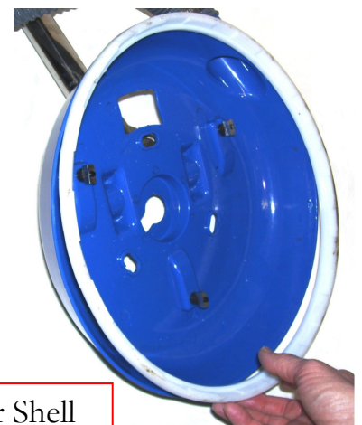
Remove the Brush Ring or Hard Boot
