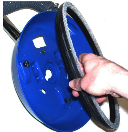
Remove the Brush Ring or Hard Boot
