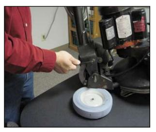
Figure 6-9. Tighten Setscrew
