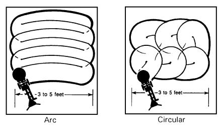
Figure 4-4. Correct Cleaning Patterns
