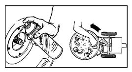
Figure 6-7. Lubricate Shaft and Re-install Head Assembly
