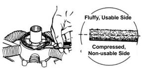
Figure 9-1. Carefully Pry Seal Up and Lift Out
