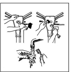
Figure 6-1. Remove Nut/Inline Filter
