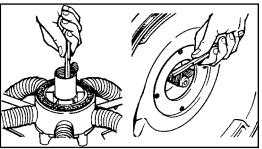
Figure 6-5. Clean Off Debris from Gear Box Shaft
