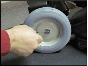
Figure 6-8. Remove Retaining Clip with Screwdriver
