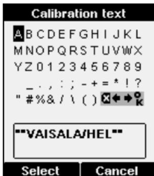
8. Select menu item **[5] Note** to edit the calibration info text that is stored in the probe. Edit the text using the select button and arrow keys. When done, select the OK character in the bottom right corner to save the changed text.
