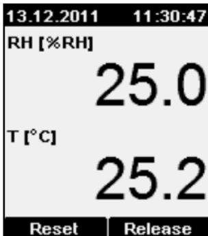
When the screen is held, the top of the display displays the current date and time. This is useful when you want to record the current data (take a photograph or write it down).
