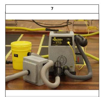
If using an Interceptor HEPA filter, attach the Main Y to the end of it's AIR IN hose and to the panel hose. You may now tape the Vac-It Panels down to the floor (test tape to be used in a hidden location first to prevent finish damage).
