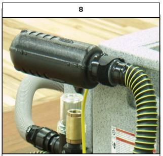
Use the provided velcro loop (power cord strap) to secure temporarily keep the Silencer up from the floor. The hot air from the AR OUT Main hose can cause damage to the flooring materials.
