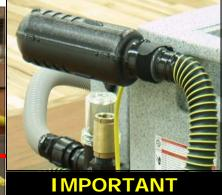
Due to probable high heat output, the Silencer should be elevated from surfaces that could be damaged by heat. Attach the Silencer with the velcro strap while in operation to hold in elevated position. The strap holds the cord for travel. Place the HP on a blanket to protect floors (many floors do not require refinishing.)
