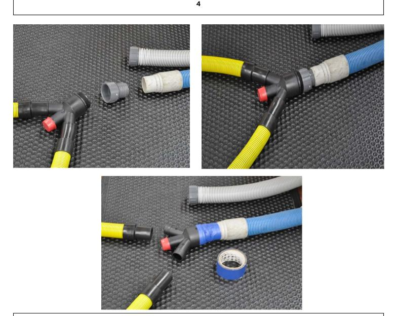
Temporarily attach the Main W with a HB300 (sold separately). Insert the barbed end into the end of 2" truckmount/portable suction line. If you do not have a HB300, use tape to temporarily seal the Main W to the end of the extraction line.
