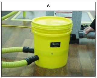
After you have finished extracting, we recommend the use of the WS for the first 24 hours. This helps catch any remaining hidden pockets of moisture that might still be migrating (with the help of the HP unit).
