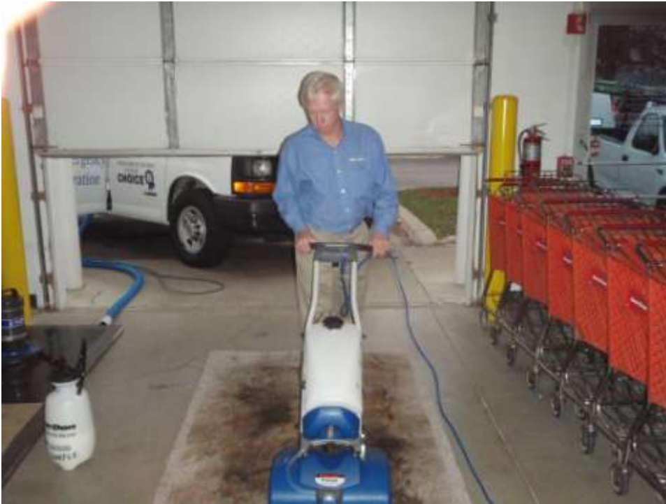
Agitation with a Counter-Rotating Brush system.
